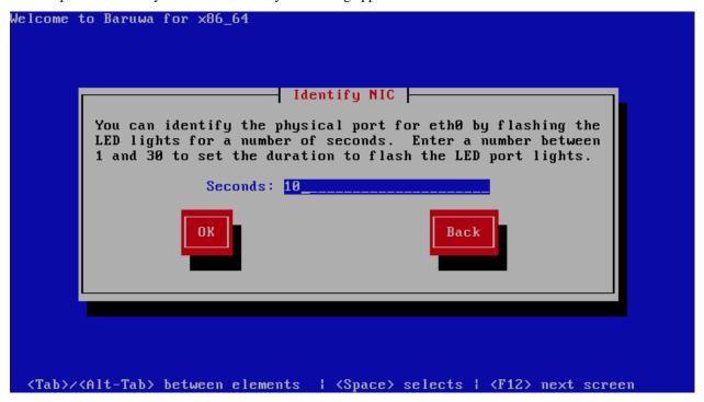
The sockets of most network devices feature an activity light (also called a link light) — an LED that flashes to indicate that data is flowing through the socket. The installer can flash the activity light of the network device that you selected in the Networking Device dialog for up to 30 seconds. Enter the number of seconds that you require, then press OK. When the installer finishes flashing the light, it returns you to the Networking Device dialog.
