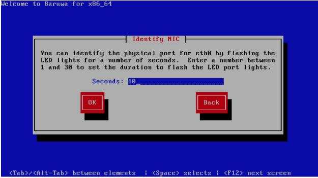
The sockets of most network devices feature an activity light (also called a link light) — an LED that flashes to indicate
