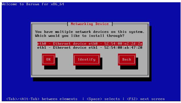
If you are not sure which device in the list corresponds to which physical socket on the system, select a device in the list then press the Identify button. The Identify NIC dialog appears.
