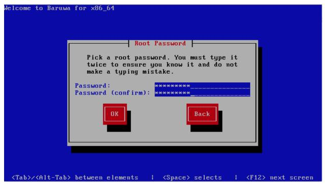
The installation program prompts you to set a root password for your system. You cannot proceed to the next stage of the installation process without entering a root password.
