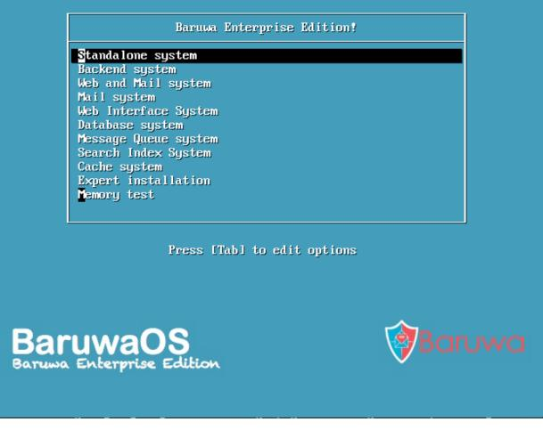
The following boot menu options are available, these options are install profiles you need to select specific profile you would like to install. The default profile is Standalone which installs the full Baruwa Enterprise Edition system to a single server.
