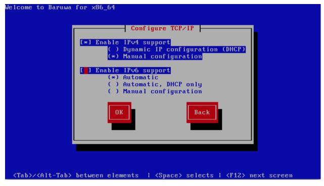
The installer prompts you to provide the details in the Manual TCP/IP Configuration dialog:
