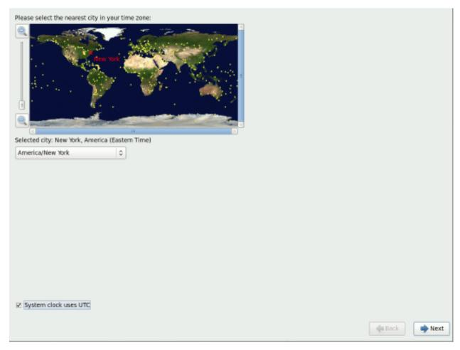
Select System clock uses UTC. The system clock is a piece of hardware on your computer system. Baruwa Enterprise Edition uses the timezone setting to determine the offset between the local time and UTC on the system clock. This behaviour is standard for systems that use UNIX, Linux, and similar operating systems.
