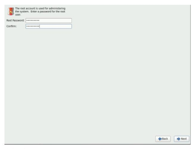
The installation program prompts you to set a root password for your system. You cannot proceed to the next stage of the installation process without entering a root password.
