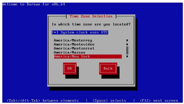
Select System clock uses UTC. The system clock is a piece of hardware on your computer system. Baruwa Enterprise Edition uses the timezone setting to determine the offset between the local time and UTC on the system clock. This behaviour is standard for systems that use UNIX, Linux, and similar operating systems.
