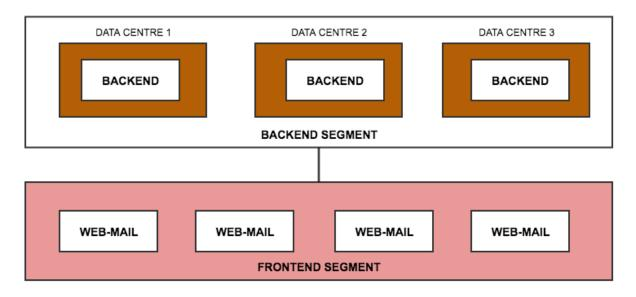
**Note: NOTE:** The smallest cluster that can be created is based on the Single Backend Hybrid Frontend topology and is made up of a clustered frontend and none clustered backend. The number of devices in this cluster is three (3). Two (2) frontend and one (1) backend.
